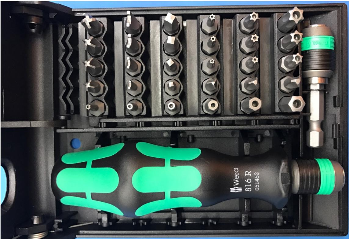
In such cases a “security bit set” is useful for field deployment, but care should be taken to not to damage a tamper-resistant fastener with the use of an incorrect bit.
