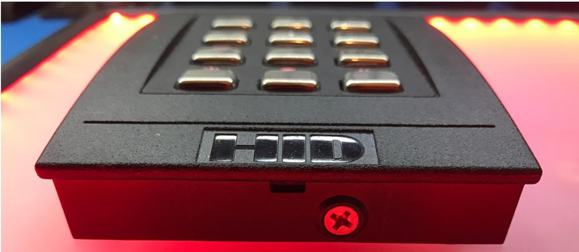
Once the fastener is removed, the reader may usually be removed by tilting it away from the wall using the side opposite the fastener as a hinge.
