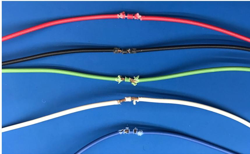
**Following removal, the wire insulation will be damaged. Insulating tape must be applied to the wiring to prevent accidental short-circuits.**
